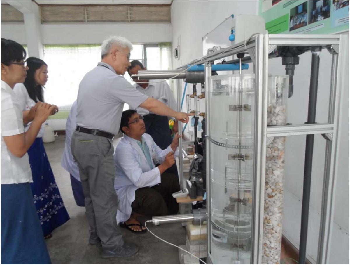
Figure (5) Experiments using Water Flow-rig for simulation of Chemical Reactor System
